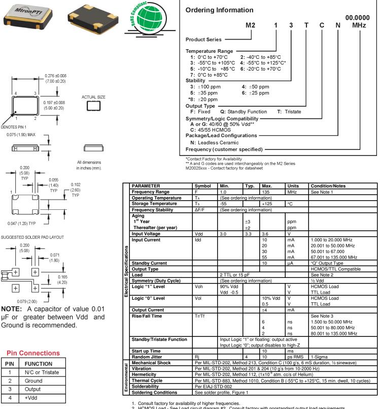
HCMOS Load - See Load circuit diagram #2. Consult factory with nonstandard output load requirements.
